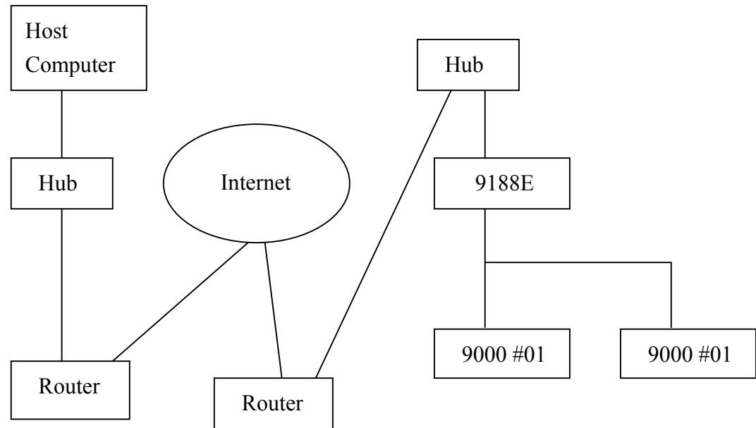
**Fig1.1 Simple Structure of EX9188E Network**
